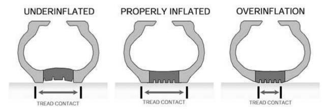
Are your tyres set at the optimum inflation? Chances are they are anywhere from 8psi to 18psi less than recommended. The most common way of damaging tyres is improper inflation. Low air pressure causes tyres to experience irregular treadwear as well as poor vehicle handling and traction. Under inflated tyres can build up excessive heat and blow out without warning.
